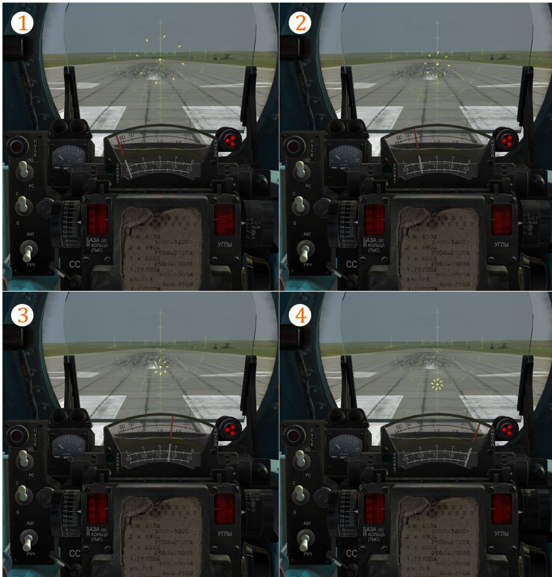
Image 10.5: Illustration of the relation between the distance (introduced with throttle rotator) and piper size and intercept angle.
