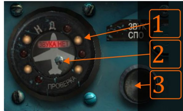
Image 10.10: 1 - flashing lights (“eyes”), white - for day, red - for night; 2 - self test button; 3 - sound volume knob.
