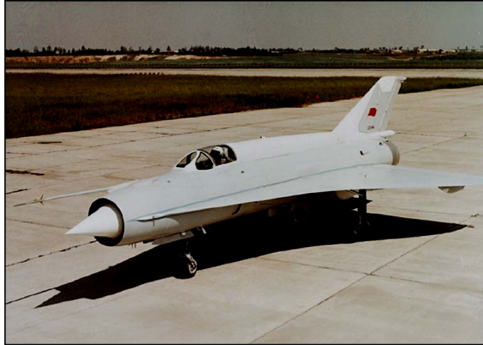
1961: MiG-21I "Analog", test-bed for research and development of Tu-144 passenger airplane wing
