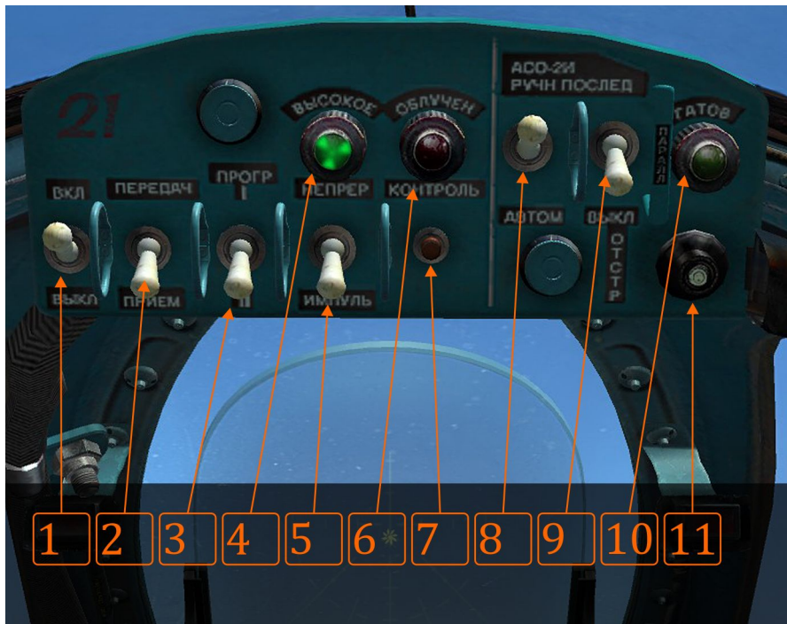
Image 10.17: SPS control box
