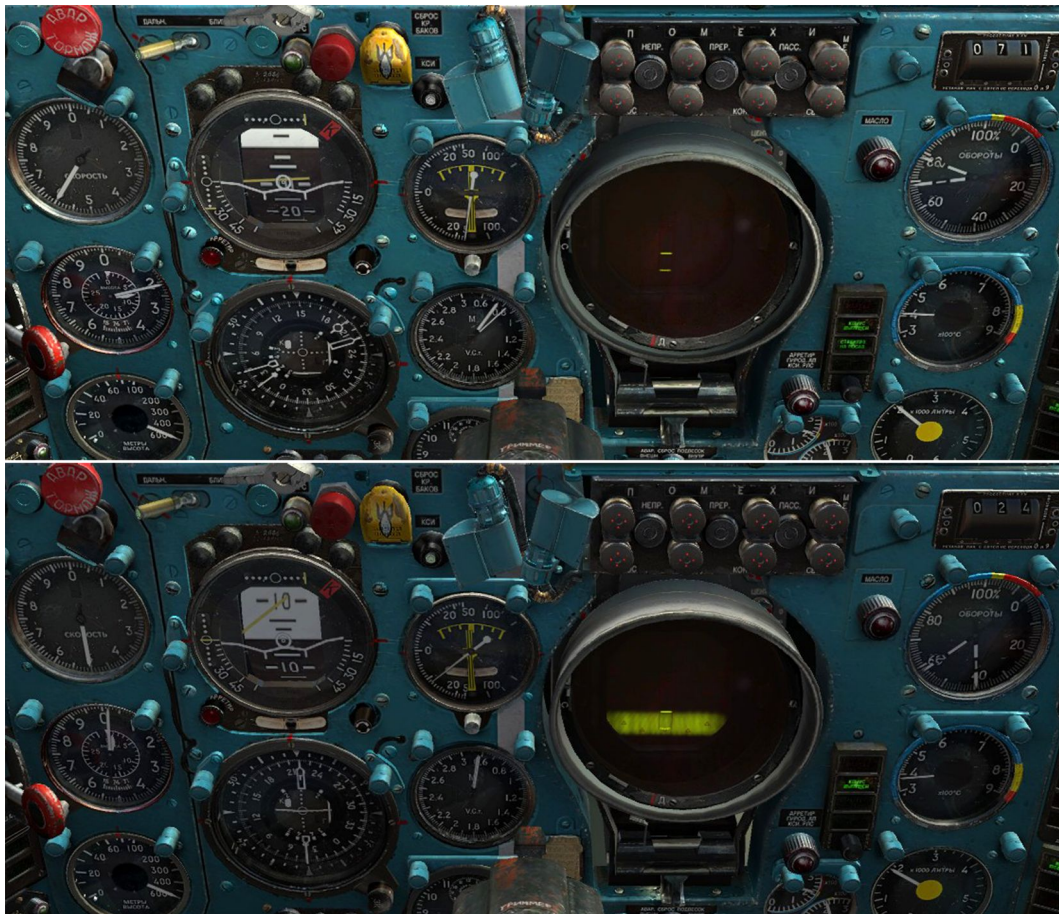
Image 9.12: Upper image shows aircraft at 71km from RSN station, while in CLOUDS PENETRATION mode. Note the glide path is below aircraft (glide needles) while vertical speed is within recommended by glide director needle (yellow needle on KPP). On lower image same aircraft is 24km from RSN station, on glide path and currently descending with greater than recommended vertical speed.
