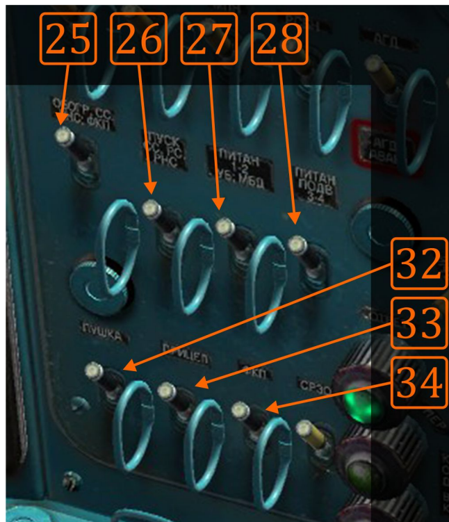
Image 10.1: Weapons activation interface on right-vertical panel.
