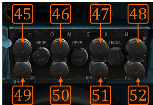
Image 10.8: Radar countermeasures and auxiliary control panel.
