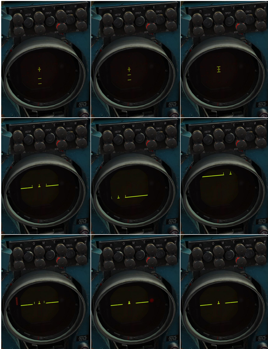
Image 10.7: illustration of radar self-test pattern
