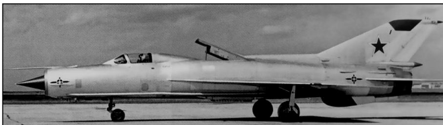
1966: MiG-21PD, experimental aircraft with short take-off and landing to develop lift engines of MiG-23PD aircraft
