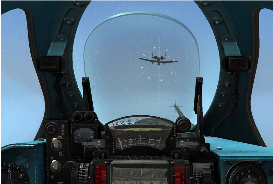
Image 10.15: Attack using the internal gun and ASP in automatic gyro mode (fixed distance 300m).
